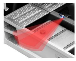
The sensor is positioned so that the harness extends beyond the vehicle's outline in order to prevent a break-in even before it occurs. To do this, during installation, the height of the harness and its maximum range must be adjusted using the control unit's Test mode (see "Perimeter Beam Adjustment").
